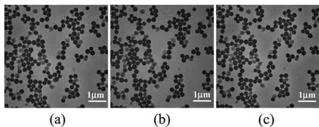
**Fig. 7** *In situ* TEM images taken from silica-encapsulated bismuth nanoparticles (a) before annealing, (b) at approximately 300 °C, and (c) after solidifying.
