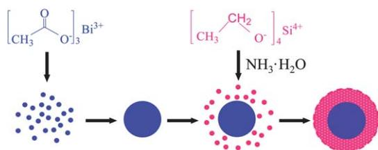
**Fig. 1** Illustration of synthesis and encapsulation of silica-encapsulated bismuth nanoparticles.
