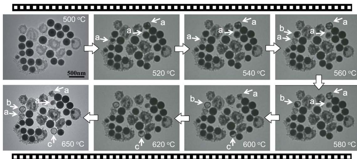
**Fig. 9** A series of *in situ* TEM images recorded from silica-encapsulated bismuth nanoparticles, where some leakages of bismuth core materials were indicated with arrows “a”, “b” and “c”.
