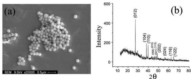
**Fig. 2** (a) Scanning electron microscope image of bismuth nanoparticles deposited on silicon wafer. (b) X-Ray diffraction spectrum of bismuth nanoparticles.
