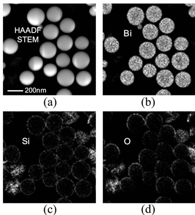
**Fig. 8** (a) HAADF-STEM image taken from silica-encapsulated bismuth nanoparticles after *in situ* TEM annealing, and the corresponding EDS elemental mapping results for (b) Bi, (c) Si, and (d) O, respectively.
