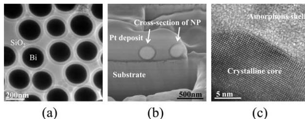
**Fig. 5** (a) TEM image taken from silica-encapsulated bismuth nanoparticles; (b) cross-sectional image of silica-encapsulated bismuth nanoparticles performed in a FIB microscope; (c) high-resolution TEM image taken at the interface between silica shell and bismuth core.
