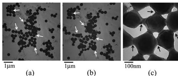
**Fig. 4** *In situ* TEM images taken from (a) as-synthesized bismuth nanoparticles, (b) the bismuth nanoparticles after annealing, and (c) the sintering necks formed between bismuth nanoparticles after annealing.
