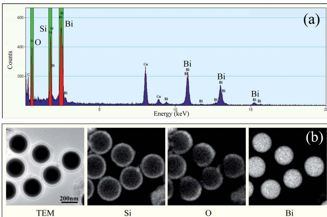
**Fig. 6** (a) X-Ray energy dispersive spectrum collected from silica-encapsulated bismuth nanoparticles, where the energy peaks of elements Si, O and Bi were indicated. (b) TEM image taken from silica-encapsulated bismuth nanoparticles and the corresponding EDS elemental mapping results for Si, O and Bi, respectively.
