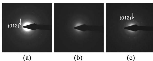
**Fig. 3** Electron diffraction patterns taken from bismuth nanoparticles at a temperature of (a) approximately 23 °C, (b) 272 °C, and (c) 167 °C, respectively, by *in situ* transmission electron microscopy.
