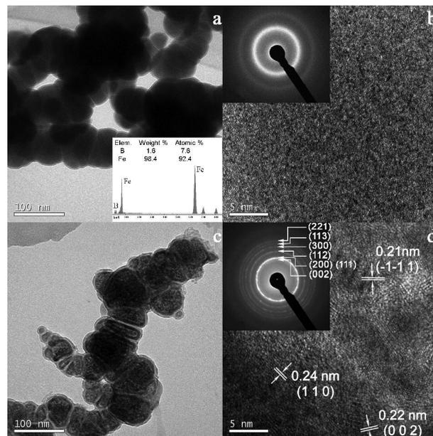
**Figure 2.** TEM image of the amorphous iron precursor and final product nitrided at 573 K. (a) Ball-like TEM image of the iron precursor (with EDAX result inner). (b) The short-range order (not long-range order) structure of amorphous iron (with SAED image inset). (c) TEM image of final product  $\epsilon$ - $\text{Fe}_{2-3}\text{N}$ . (d) Crystalline lattice structure of  $\epsilon$ - $\text{Fe}_{2-3}\text{N}$  (with SAED image inset).
