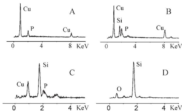
**Figure 4.** EDX spectra of copper-phosphor micro/nanowire after the first (A), second (B) and third (C) draw cycle, and the comparison to that on a near-by glass region (D).
