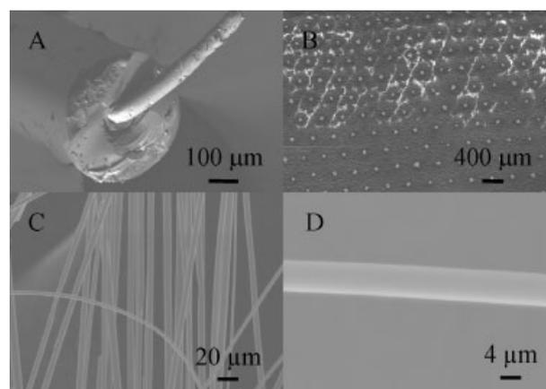
**Figure 2.** SEM images of glass encapsulated copper-phosphor microwire (A) and the large array of the copper-phosphor microwires (B) after the first draw cycle. Copper-phosphor microwires (C and D) made in the second drawing, where the glass coating is removed before imaging.
