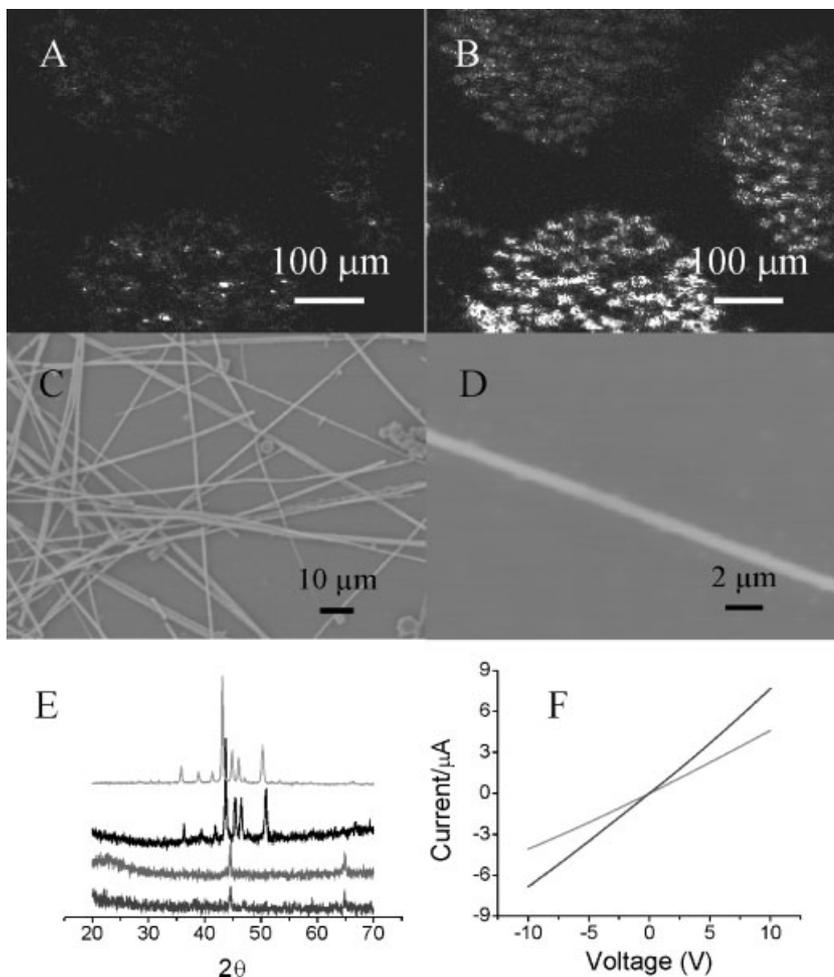
**Figure 3.** The distributions of phosphor (A) and copper (B) on a flat plate after the second draw-cut-stack cycle obtained using SIMS; SEM images of copper-phosphor nanowires obtained in the third draw cycle after removing glass coating (C and D); XRD curves of the copper-phosphor powder, and those obtained after the first, second and third draws (from top to bottom) (E); the current-voltage relation measured across an array of microwires (F).
