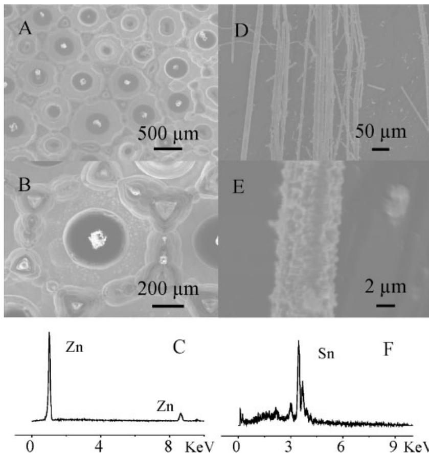
**Figure 5.** SEM images of zinc microwires embedded in glass matrices (A and B) and the according EDX spectrum (C); SEM images of tin microwires after removing the glass coating (D and E) and the according EDX spectrum (F).
