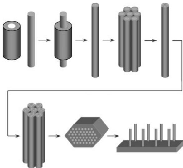
**Figure 1.** Scheme of making aligned micro/nanowires using fiber-drawing nanomanufacturing.
