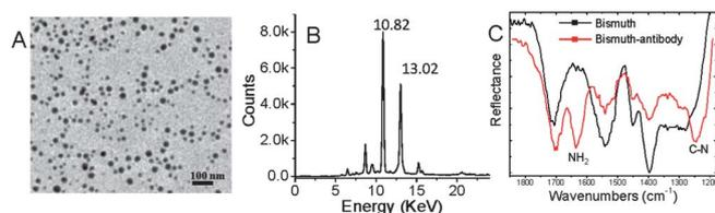
**Fig. 2** Synthesized bismuth nanoparticles and their conjugation with antibodies. TEM image (A) and XRF spectrum (B) of bismuth nanoparticles; (C) FTIR spectrum of unmodified and antibody-functionalized bismuth nanoparticles.
