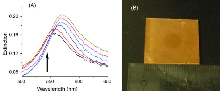
**Fig. 3.** (A) The extinction spectra of gold nanoparticles after exposing to DNT vapor, where the curves are taken at 0, 5, 10, 15, 20 and 25 s (bottom to up), respectively; (B) a micrograph of a circle pattern not exposed to DNT.
