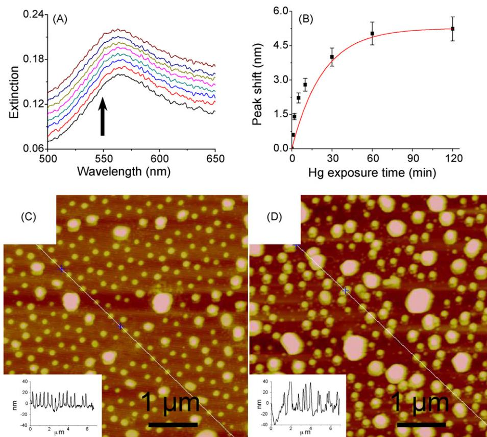
**Fig. 4.** The peak shifts of gold nanoparticles after exposed to 15 ppm mercury vapor (A), where the curves are taken at 0, 1, 2, 5, 10, 30, 60 and 120 min (bottom to up), respectively; (B) the magnitude of peak shifts at different exposure time; AFM images of nanoparticles before (C) and after (D) exposing to mercury for 120 min, where insets show the according cross-section profiles.
