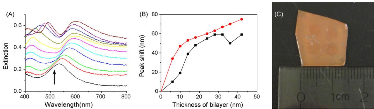
**Fig. 2.** (A) The UV-visible extinction spectra of silver nanoparticle array with 0–10 bilayers of PAH/PAA (bottom to top), respectively; (B) the experimental (square) and simulated (circle) peak shifts as functions of numbers of bilayers, respectively; (C) a micrograph of circle patterns that have been covered by three bilayers of PAH/PAA.
